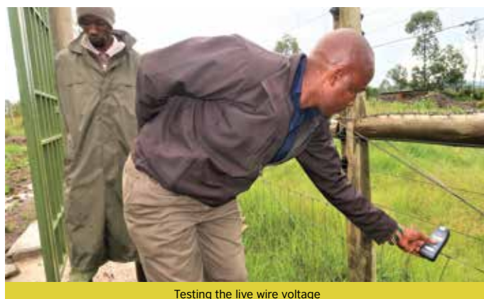
Testing the live wire voltage
